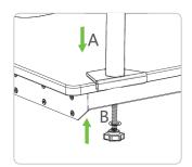
Place the column (A) then tighten the bolt (B) underneath, secure the main column.
