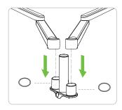
Slide the nylon washers onto the dual arm connector then position both arms onto connector.
