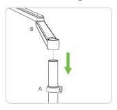
A Slide the retaining ring (A) onto the column, then insert the double section arm (B) onto upright column.
