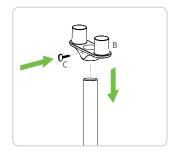
5 Insert the dual arm connector (B) into the post. Adjust the appropriate position then tighten the screw (C).
