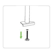
Remove the base screw from column.
