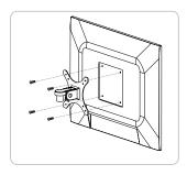
Place VESA bracket in position on back of the monitor with lip facing up, attach using 4 screws provided.
